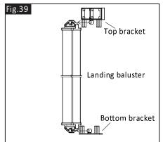
Place the balusters into the baserail groove and carefully lower handrail assembly complete with wall connector inserted but not fixed, onto top baluster bracket so it is fully located into the handrail groove (Fig.40).
