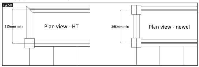
It is possible to reduce minimum centres by 30mm when using HT, and 60mm when using newel, by cutting off locator arm on the landing connector (IMLC) as the locator arm is not used in this particular configuration.
