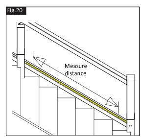
To calculate the number of balusters required, divide distance by 148.5. Round the figure up to next whole number. Divide the distance by the whole number to give centres for remaining baluster locations.
