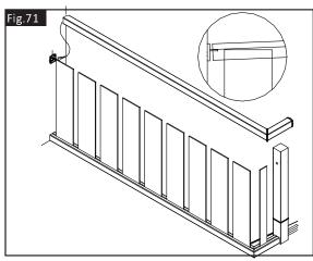
Once the handrail is fully located on top of the glass panels, secure in place by inserting the bolt and washers through the newel into the landing connector (IMLC) and tighten.
