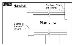
Fix HT connector to the mitred end of the rail by offering the connector over the rail, ensuring the locator arms are up against the top of the groove. Pilot drill through locating arm to a depth of 15mm and secure with screws supplied. Fix other mitred rail end into HT connector and repeat.
