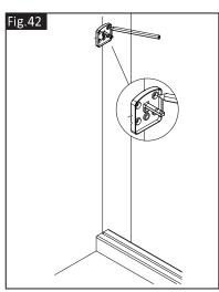
For the landing connector, run a line from mark to opposite face of the newel. Mark the centre of the newel and drill a 16mm diameter counter bore hole to a depth of 20mm and a 10mm diameter through hole (See Fig.15 & Fig.16).
