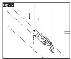
To fix top bracket, ensure that baluster is fully pushed into handrail and is perpendicular. Pilot drill through back hole to a depth of 15mm using 3mm diameter long series drill bit and secure with 44mm screw supplied. Use piece of tape on drill bit to act as depth gauge (Fig.27).
