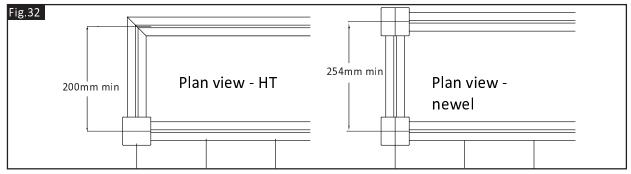
It is possible to reduce the minimum centres by 30mm when using the HT and 60mm when using the newel by cutting 30mm off the locator arm on the landing connector (IMLC) as the arm is not used to fix the rail in this particular configuration.
