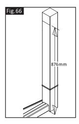
Run a mark to the opposite face of the newel. Mark the centre of the newel and drill a 16mm dia counter bore hole to a depth of 20mm and a 10mm diameter through the hole (see Fig.16 on page 4).
