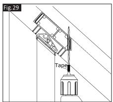
To fix final two balusters, line bottom bracket central to mark on tape ensuring that back hole in bottom bracket lines up with pilot drill hole and fix with screw supplied. To fix top of baluster, pilot drill through front hole in top bracket and fix using screw supplied. A summary example of which bracket holes to use to fix balusters and also the sequence, can be found in (Fig.30).
