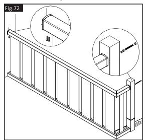
Insert the handrail timber fillets between the glass panels into the groove, pilot drill and fix with 50mm long No 6 screws.
