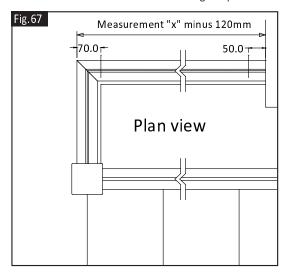
Divide the distance by 250 and round down to the whole number, this gives the number of panels required. Multiply the number of panels by 200. Subtract this number from the original measurement (measurement less 120mm). Divide by number of panels less 1 (to give gap sizes)
