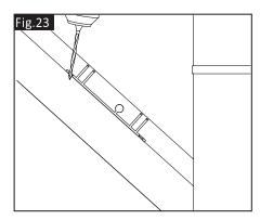
Remove bracket and drill vertically down to a depth of 30mm (Fig.24).
