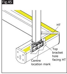
To calculate locations for rest of balusters, measure distance between the 100mm and the 115mm marks and divide by 118. Round figure up to next whole number. Divide distance by whole number to obtain baluster centres.
