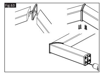
Slide the wall connector (IMWC) over the end of the rail to be fixed to the wall and drill 2 x pilot holes through the locator arm but do not fix at this stage (Fig.64).
