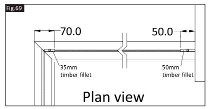
Starting from one end of the baserail, apply a bead of clear silicone 200mm long and insert the glass panel into the groove on top of the silicone, ensuring the edge of the panel is fully up against timber fillet.
