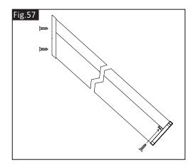
To fix the handrail to the newels, carefully offer the handrail onto the intermediate connectors so that the top rake connector is touching the top newel.
