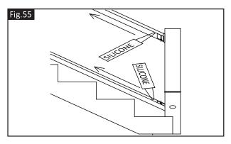
Insert the glass panel into the groove and up against the previously installed fillets. Place another set of top and bottom fillets, pilot drill and secure. Depending on how many panels are used and the gaps between them, you may have to insert the last 2 panels into the groove first before installing the fillets.
